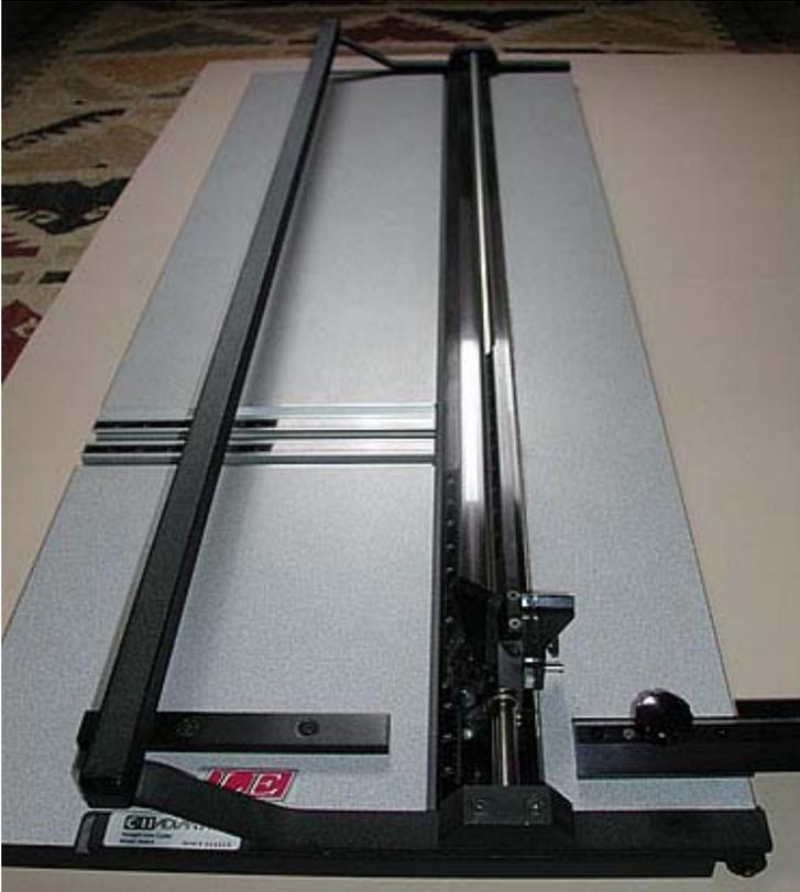
I acquired a C&H Advantage Pro table mat cutter when my sales volume increased to the point that using the Dexter was both time consuming and impractical. A table mat cutter will both speed up mat cutting and provide greater precision and reliability.
