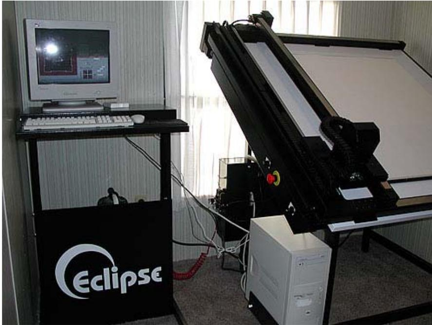
Such a machine combines three technologies to cut mats in ways that hand-operated mat cutters can never dream of: a computer running mat-design software, an x-y axis motion controller connected to two micro stepping motors, and an air compressor.
